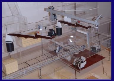
model of working deck (scale 1:50) with all lifting devices (cranes, frames, beams and winch room) allows to simulate all desired functions and helps to find weak points as well as necessary changes
